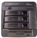
Rotatable cage for ODD or storage kits
