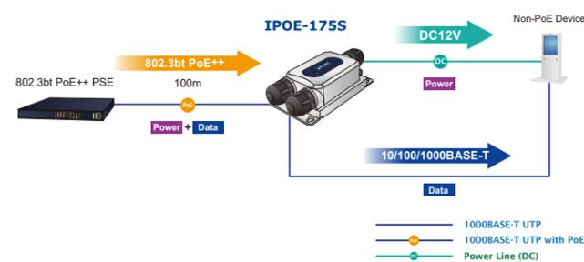
**Step 1:** Connect attached **"Power cable with 2-pin terminal block"** to the **"DC Out"** port of IPOE-175S Splitter.
