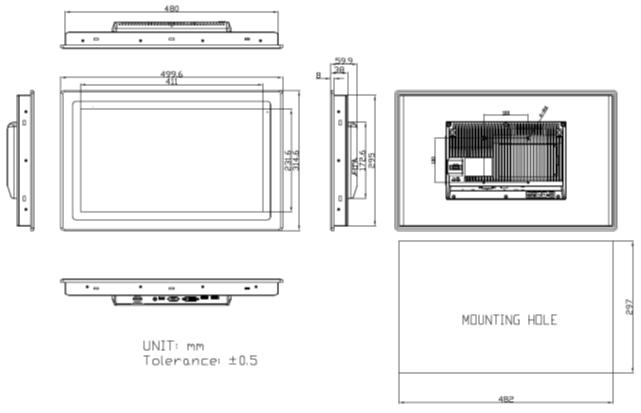
Figure 1.5: Dimensions of ARCDIS-118APRG(H)
