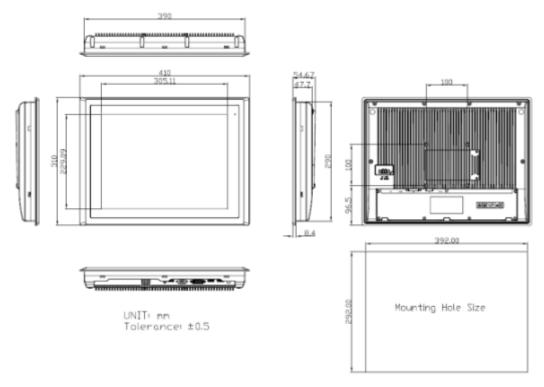
Figure 1.2: Dimensions of ARCDIS-115APRG(H)
