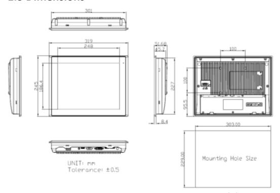
Figure 1.1: Dimensions of ARCDIS-112APRG(H)
