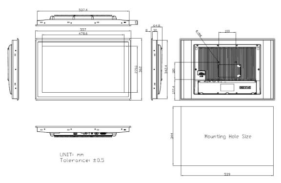
Figure 1.7: Dimensions of ARCDIS-121APRG(H)
