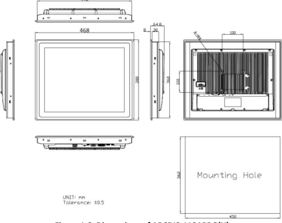
Figure 1.6: Dimensions of ARCDIS-119APRG(H)
