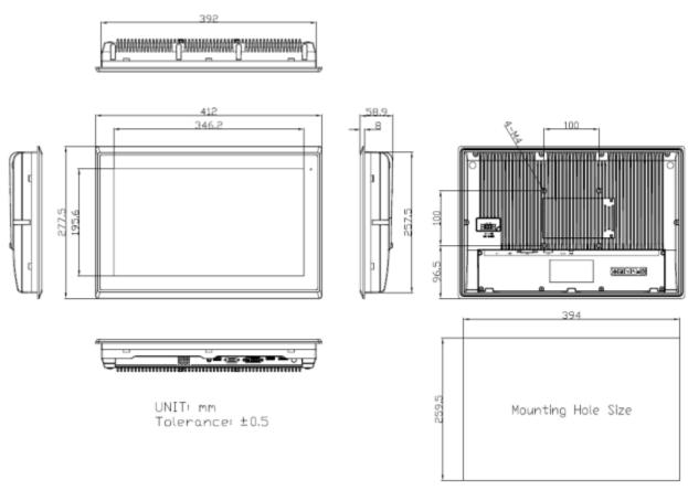
Figure 1.3: Dimensions of ARCDIS-116APRG(H)
