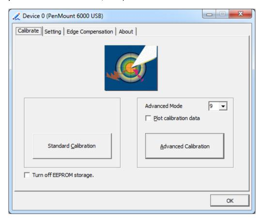
**NOTE:** Recommend to use a stylus during Advanced Calibration for greater accuracy.
