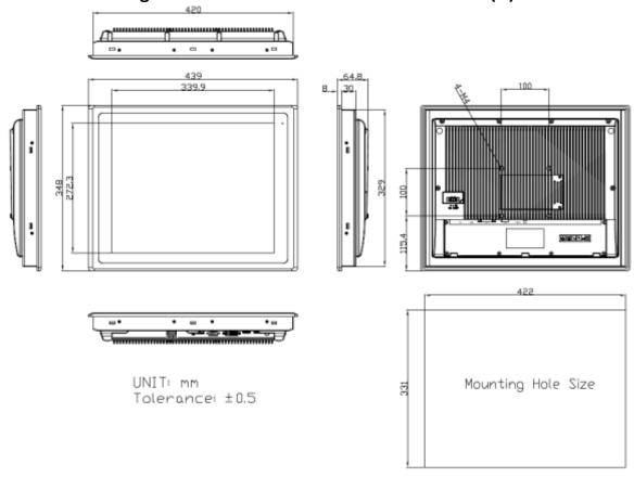
Figure 1.4: Dimensions of ARCDIS-117APRG(H)
