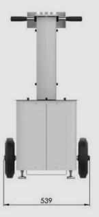
Weight ex. Robot: 45 kg, the EasyWork has a horizontal Robot Consule.
