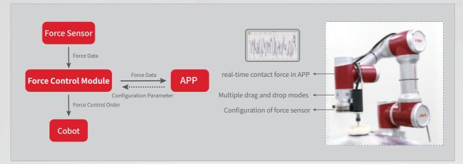
Schematic diagram of force control function
