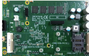
Great expandability with 2 PCI Express Mini Card slot + 1 SIM card slot
