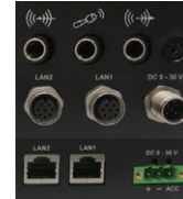
Optional I/O ports for audio, LAN jack type and DC-in jack type
