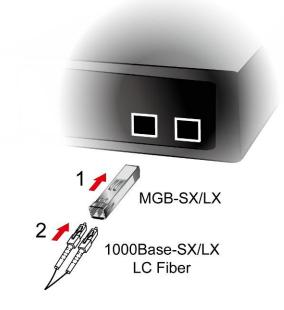
Figure 2-1-2e Plug in the SFP transceiver
