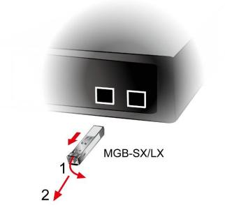
Figure 2-1-2f How to Pull Out the SFP Transceiver
