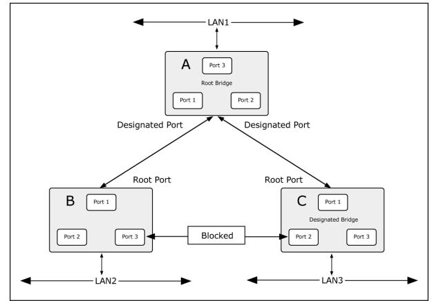
Figure 4-6-3 After Applying the STA Rules
