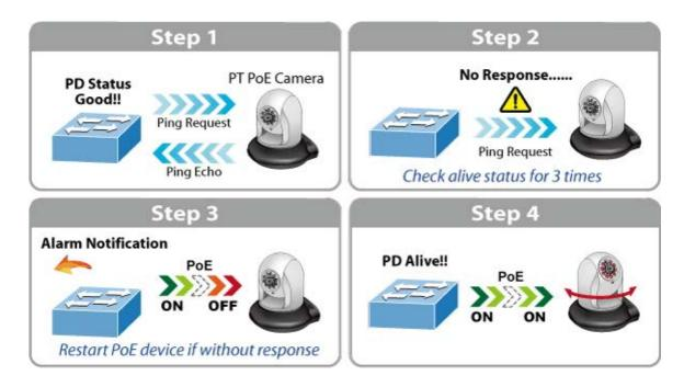
This page provides you with how to configure PD Alive Check. The screen in Figure 4-15-7 appears.
