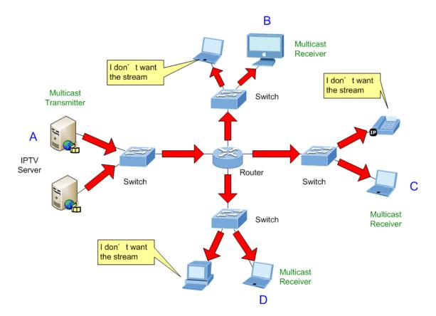
Figure 4-7-4 Multicast Flooding
