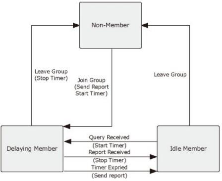
Figure 4-7-6 IGMP State Transitions
