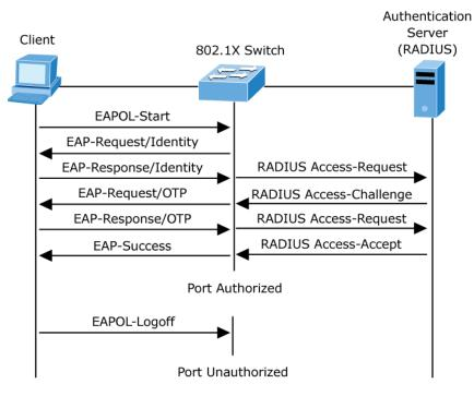
Figure 4-9-2 EAP Message Exchange
