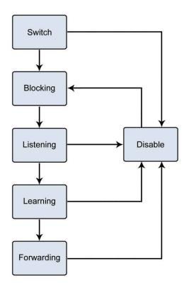
Figure 4-6-1 STP Port State Transitions
