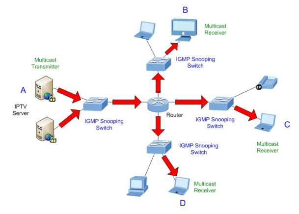
Figure 4-7-5 IGMP Snooping Multicast Stream Control
