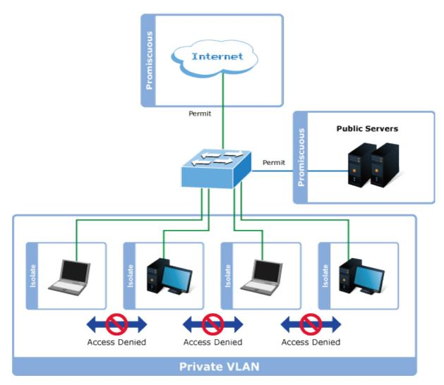
For protected port group to be applied, the Managed switch must first be configured for standard VLAN operation. Ports in a protected port group fall into one of these two groups:
