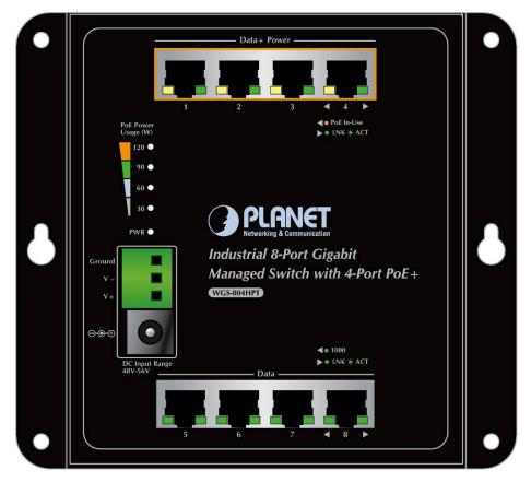
Figure 2-1-1a WGS-804HPT Front Panel
